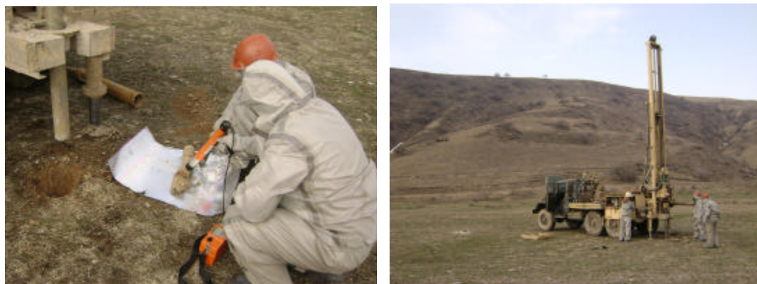
Figure 2: Kyrgyz geological staff commencing drilling and sampling tailings deposits
